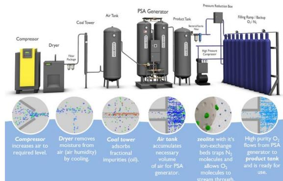
Scope of supply of a typical oxygen generation system.
